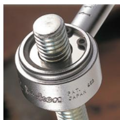
Puller for tightening stud bolts. Go-through body allows puller to grip the stud bolt at any position along the stud. Three-roller protects the bolt from damage.
