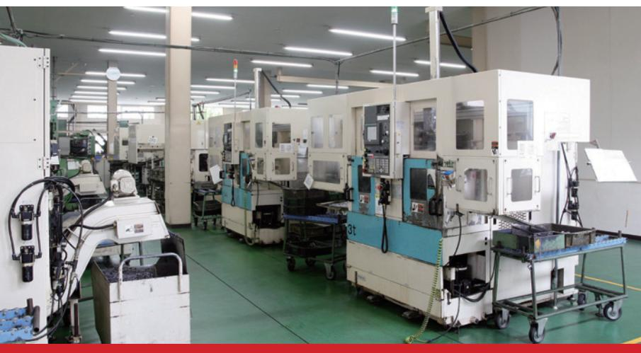
The forged steel is turned into required shapes and dimensions. The MC (Machining Center) operates with extraordinary speed and precision. The article number, size, logo, production number, and MADE IN JAPAN are marked on the products after the turning process has been completed.
