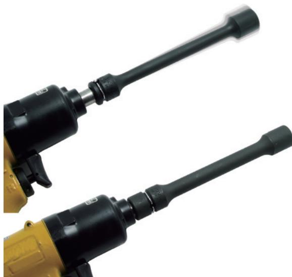
The deepened drive end of the **Sleeve-Drive** tools prevents the sometimes "wobbly" connection between pulse tool - extension - socket. An O-ring inside **Sleeve-Drive** optimizes the perfect fit of extension bars and sockets on the anvil to the effect, that the exactness of the required torque given by the pulse tool is generally improved. Further, the **Sleeve-Drive** avoids the direct transmission of vibrations on the pulse tool and finally on the operator.
