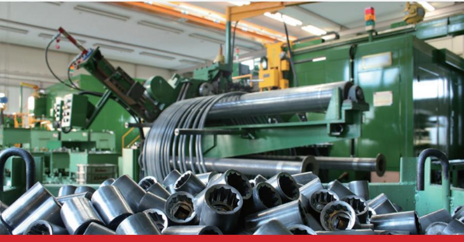
The Forming machines are used for the forging process. These machines can produce mass quantities of sockets and parts with high accuracy that ordinary drop forging machines can not achieve. However, for small production runs, ordinary forging machines are also used.
