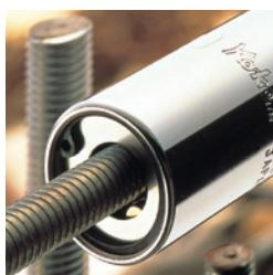
The body design was changed to hexagonal shape to minimize tolerances. This shape is also effective to lessen excessive load on cages and rollers inside the body.
