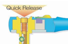
Reversible Ratchet with quick release button has less strength compared with normal ratchet due to the technical design. Make sure to use the ratchet correctly.
